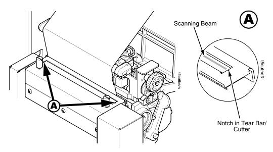
Figure 13. Aligning the Scanning Beam: Cutter Installed
